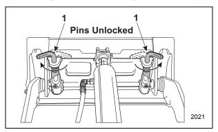
Figure 3-24 Attachment Locks in Unlocked Position
